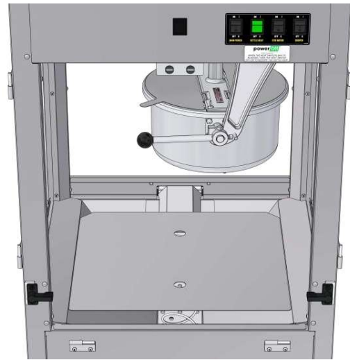
View of Tray Installed (Tray creates a level surface for kettle cleaning.)
